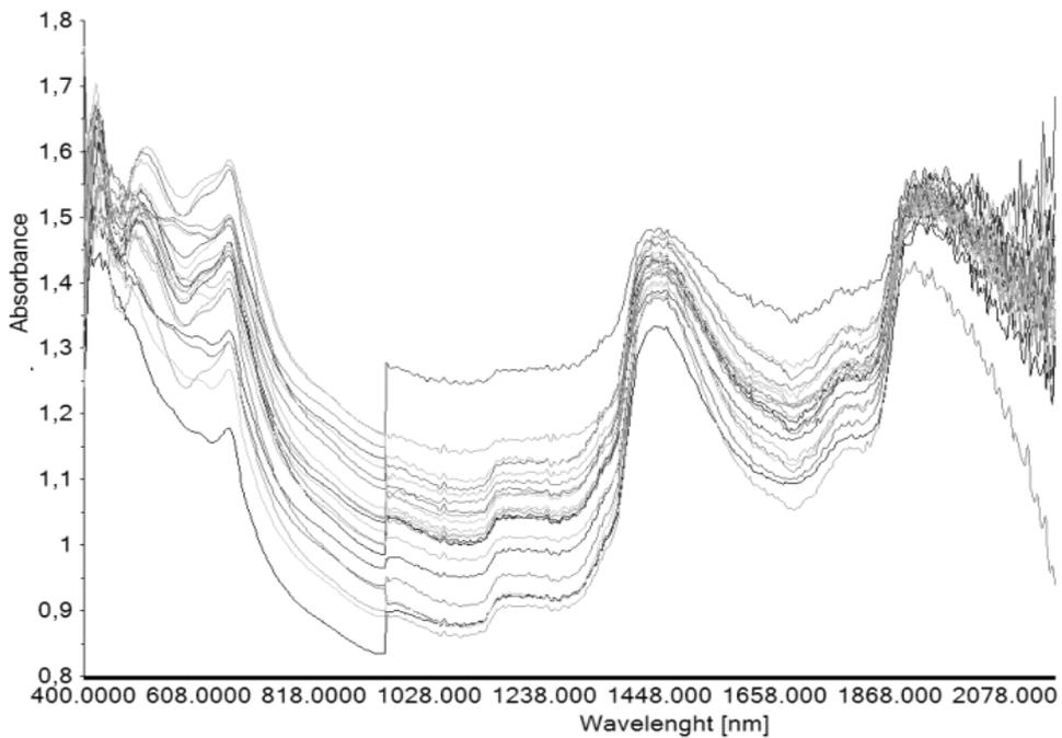
Fig. 4. Absorbance spectra for F1 samples recorded using a NIRON probe
