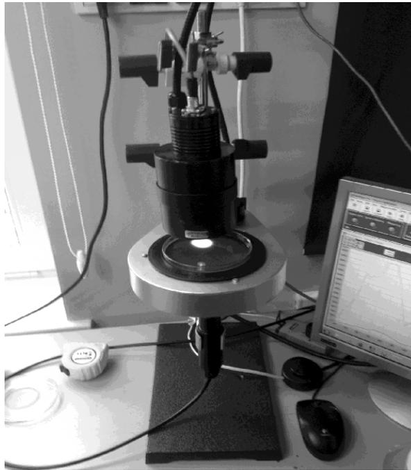
Fig. 1. A tec5 AgroSpec spectrometer applied in tests
